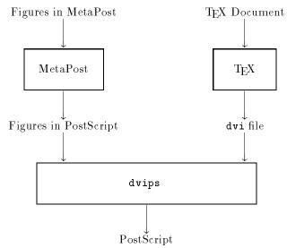
Fig. 1: A diagram of the processing for a  $T_{\! E\! X}$  document with figures done in MetaPost
