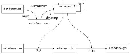
Figure 1 Compilation process of a METAPOST file
